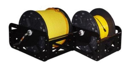
These reels will handle cables for small ROVs, camera systems, sonar equipment as well as many other applications. They are available in two drum sizes (11" x 24" and 19" x 24" both with 11 inch cores). Options included, power or manual drive, level wind, lifting bar, and an encoder for metering the cable payout.
