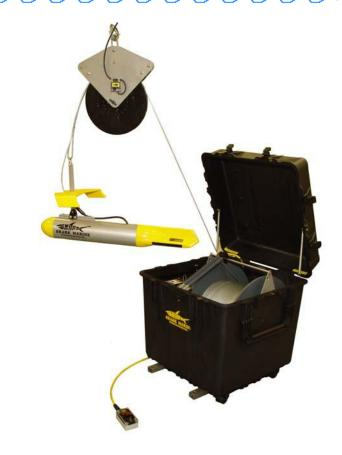
The Contained Cable Reel is designed for easy handling and storage of smaller diameter cables. It's an all-in-one tethering solution for camera systems, scientific instruments, sonar equipment and many other applications. The easily transportable unit includes a 1 Hp bidirectional variable speed drive with a maximum speed of 1 m/s, a variable gearing level wind system, slipring and a built in encoder with shive for monitoring the cable payout
