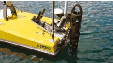
Equipped with a shell to protect the probe and cable during deployment
